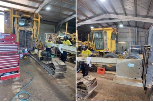
Machine breakdowns – grader blown engine, dozer roller failure. Note that all plant machinery are now repaired and in service.
